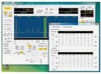
Figure 6 — *PowerSDR* offers 3 or 10 band graphic equalizers for both receive and transmit.
